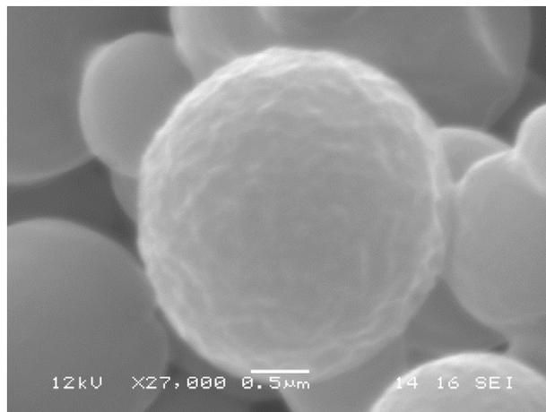
Fig. 2 SEM image of a single PUC50 microsphere; dimension bar = 0.5 µm
