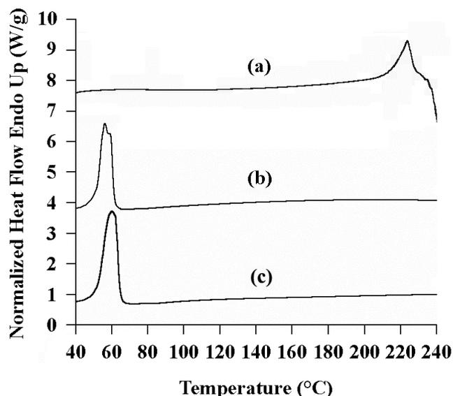
Fig. 4 DSC traces of pure PTX (a) and of the microspheres, loaded (b) and not loaded (c) with 20% PTX
