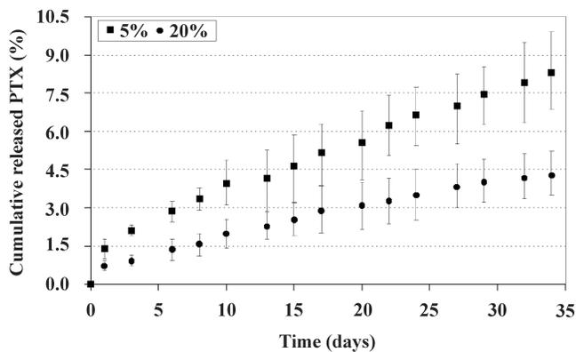
Fig. 5 Profiles of the PTX released from C27 microspheres loaded with both 5% (■) and 20% (●) PTX
