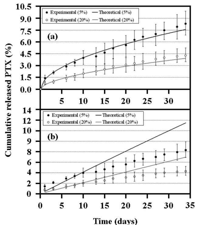
Fig. 6 Comparison between experimental and theoretical data obtained through the Peppas (a) and the Hopfenberg (b) models for the PTX released from C27 microspheres loaded with both 5% (●) and 20% (○) PTX
