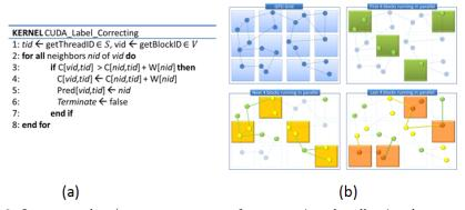
Fig. 2. Instant update/propagate strategy for computing the all-pairs shortest path problem on a GPU: (a) the GPU Kernel (b) execution example on GPU Grid. The updated distance cost is instantly reused by the subsequent block computations. This example assumes there are four streaming multiprocessors, each executing one block at a time.
